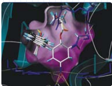
The X-ray structure of wild type tern N9 influenza virus neuraminidase (2QWK) shown with five ligands generated using RACHEL that are predicted to be active.
